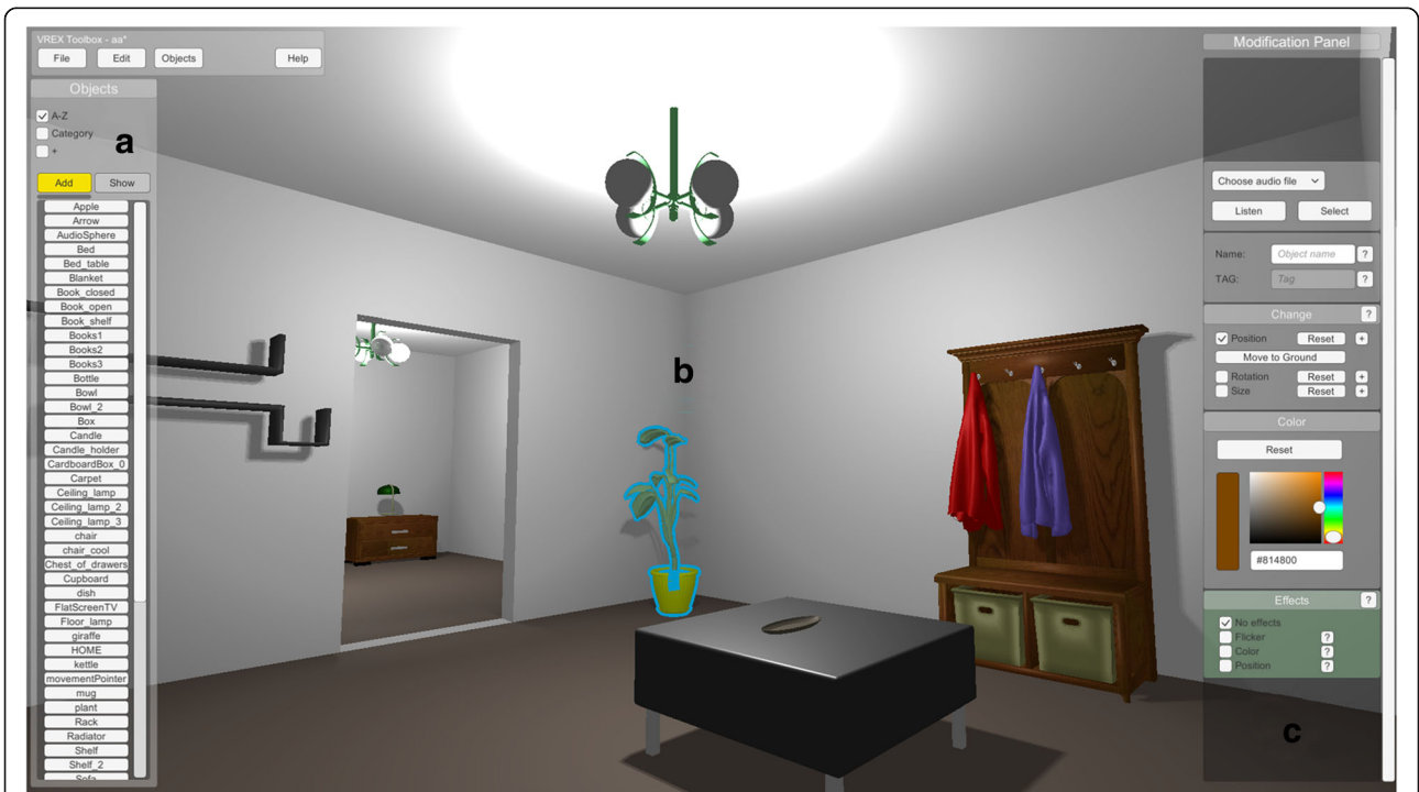
Fig. 6 The 3D editor allows to navigate and place individual objects in the scene manually (a), select objects in the environment (b) and change different properties of the chosen object, such as position, rotation, size and colour (c)
